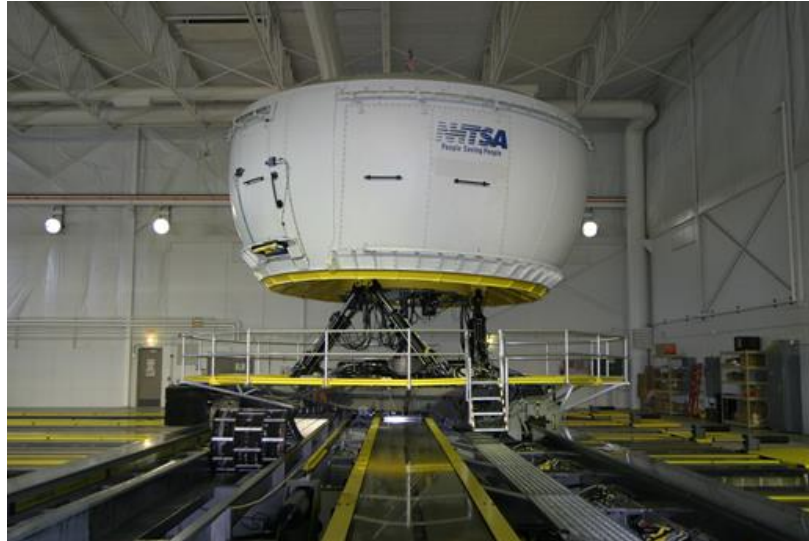
Figure 2. The NADS-1 dome exterior
