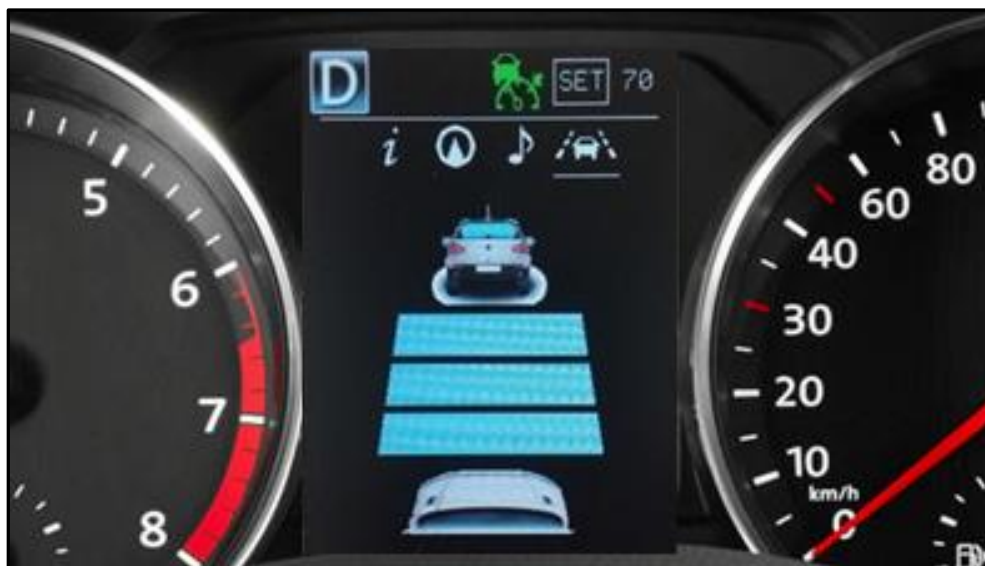
Figure 5. Close-up of ACC interface
