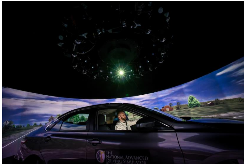
Figure 3. The NADS-1 interior with Toyota Camry cab
